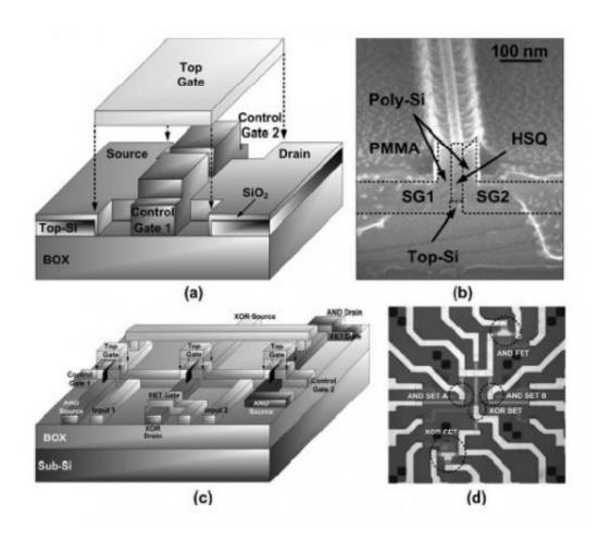
Researchers have fabricated a half-adder logic circuit with just three SETs and two FETs, compared with 20 FETs in a traditional CMOS half-adder. The new half-adder's small size and ultra-low power consumption make it promising for next-generation terabit-level nanoelectronics. Image credit: S. J. Kim, et al. ©2012 American Institute of Physics
