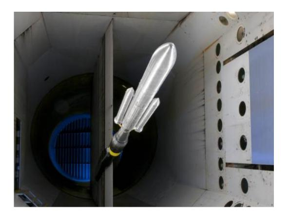
NASA's Space Launch System buffet model in NASA's Langley Researcher Center's Transonic Dynamics Tunnel. The SLS is America's next heavy-lift launch vehicle that will provide an entirely new capability for science and human exploration beyond Earth's orbit. Credit: NASA/LaRC
