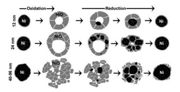
The number and location of nucleation sites of nickel metal within nickel oxide nanoparticles during their reduction with hydrogen strongly depend on the nanoparticle size.
