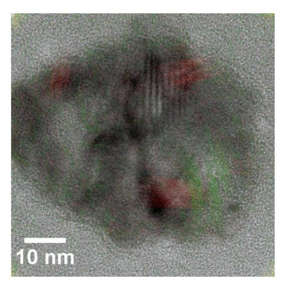
Image of a partially reduced 40 nm nickel oxide nanoparticle. The nickel region is colored red, and the nickel oxide is colored green. Click to enlarge image.
