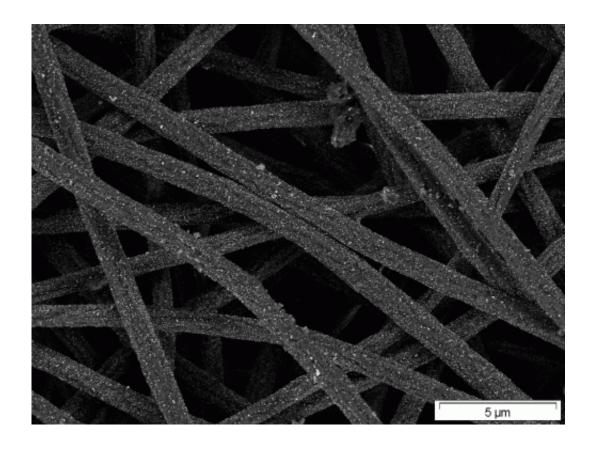
A microscope image of the membrane after the filtering. The gold particles are well dispersed. Credit: John Wiley and Sons
