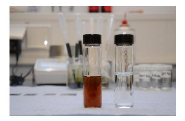
The Nanofluid with particles of gold (left) and the solution filtered (right). All metal paticles are filtered out. Credit: CAU, Photo: Claudia Eulitz
