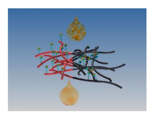
The graphic shows a membrane consisting of polymer fibres (red and black) with proteins (blue) that have activated their ability to capture all the metal nanoparticles. When the Nanofluid with metal particles (top) passes through the sieve, the proteins hold the particles. At the end, there is a liquid which is free of particles. Credit: John Wiley and Sons
