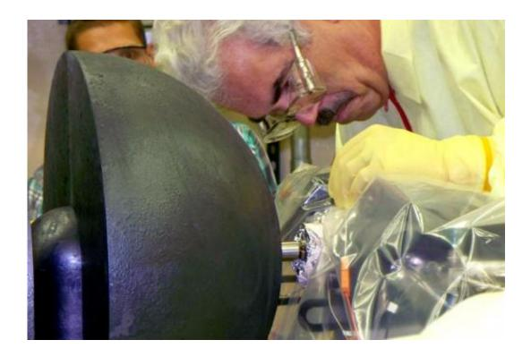
John Bounds of Los Alamos National Laboratory's Advanced Nuclear Technology Division makes final adjustments on the DUFF experiment, a demonstration of a simple, robust fission reactor prototype that could be used as a power system for space travel. DUFF is the first demonstration of a space nuclear reactor system to produce electricity in the United States since 1965.
