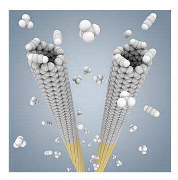
Cloning nanotubes: In this computer model, small, pre-selected nanotube "seeds" (yellow) are grown to long nanotubes of the same twist or "chirality" in a high-temperature gas of small carbon compounds. Credit: USC
