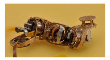
A four-segment milli-motein chain with a one-centimeter module size. Credit: MIT Center for Bits and Atoms
