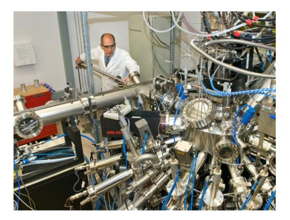
Brookhaven Lab physicist Ivan Bozovic with the molecular beam epitaxy system he uses to engineer atomically precise superconducting materials.
