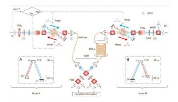
The experimental setup for quantum teleportation between two remote atomic ensembles. Credit: Bao, et al. ©2012 PNAS Early Edition
