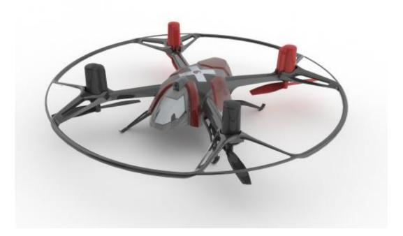
The copters can talk to each other via infrared transmitters and receivers. Team colors are automatically displayed with changing LED colors on both the craft and the controllers. The QFO Labs mission has been to take the gaming experience off a "flat <u>video screen</u> and into the physical world."
