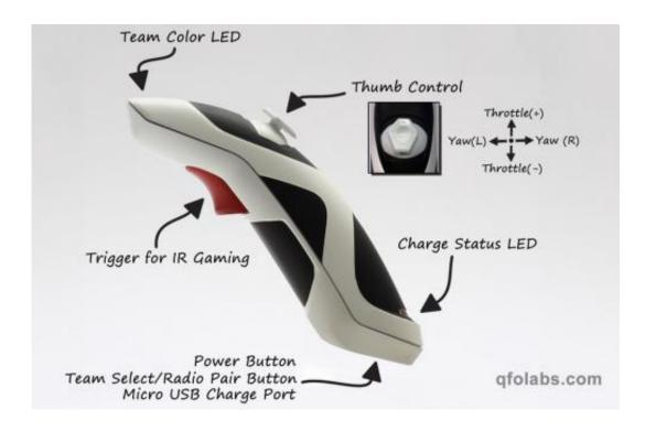
For serious tinkerers, the system's open communications protocol means being able to connect a computer up to the Mimix through the USB port to communicate wirelessly with the NanoQ to do things such as tweak control parameters, send control commands from a laptop, send customized signals out of the IR transmitter, or even connect an Arduino or camera to the auxiliary serial port on the NanoQ.
