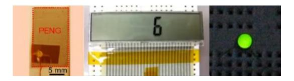
(Left) A photograph of the PENG, (center) the PENG powers an LCD for more than 60 seconds, and (right) a green LED is powered by a Li-ion battery that was charged by the PENG. Image credit: Yang, et al. ©2012 American Chemical Society
