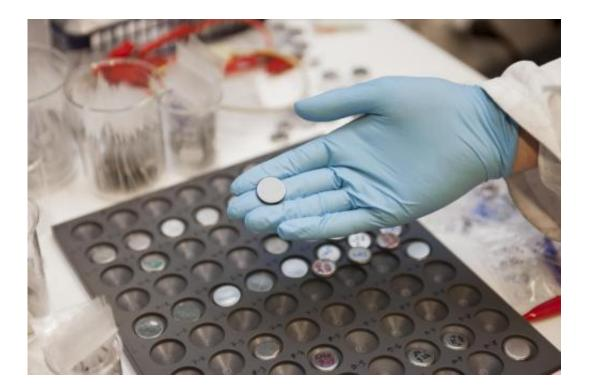
Finnish researchers found a way to significantly improve the durability of Lithium-ion batteries by covering the electrodes of lithium iron phosphate batteries with extremely thin protective layers, and by increasing the potential of lithium iron phosphate used as a positive electrode by doping. Credit: Aalto University
