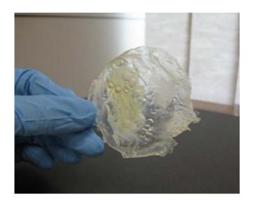
Acrylic acid-based polymers and co-polymers (pictured) can now be synthesized using free radical chemistry, thanks to new ligand–initiator type molecules. Credit: 2012 A\*STAR Institute of Chemical and Engineering Sciences
