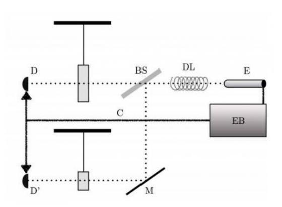
Set up of suspended blocks showing (dotted) the alternative paths for the photon. E is the single-photon emitter, D and D' are the single-photon detectors. BS denotes the beamsplitter and M the mirror. DL is the fi ber optics delay line, and EB are the electronics that trigger D and D' through cable C. The optical elements to widen the beam before and focus it after each block are left out for clarity. In the real experiment the blocks would hang side by side. Credit: arXiv:1211.3816 [gr-qc]
