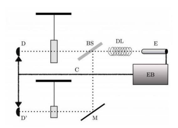
Set up of suspended blocks showing (dotted) the alternative paths for the photon. E is the single-photon emitter, D and D' are the single-photon detectors. BS denotes the beamsplitter and M the mirror. DL is the fi ber optics delay line, and EB are the electronics that trigger D and D' through cable C. The optical elements to widen the beam before and focus it after each block are left out for clarity. In the real experiment the blocks would hang side by side. Credit: arXiv:1211.3816 [gr-qc]
