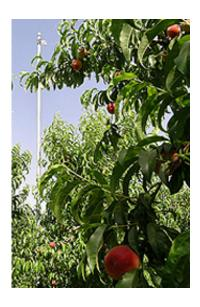
Infrared thermometer mounted on a pole for measuring peach tree canopy temperature under regulated deficit irrigation. Stressed leaves have a higher temperature than nonstressed leaves. Photo by Dong Wang
