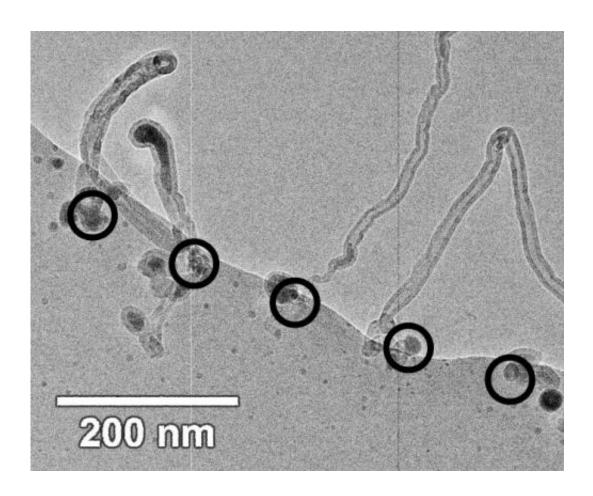
Bright field transmission electron micrograph showing carbon nanotubes grown from an array of equally-sized iron catalyst particles created by electron beaminduced decomposition of a diiron nonacarbonyl precursor.
