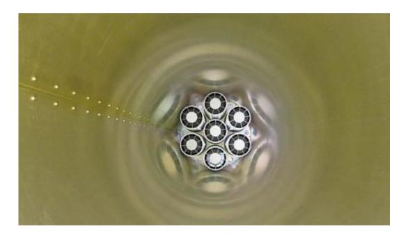
Looking down the telescope tube on FOXSI the Focusing Optics X-ray Solar Imager reveals state-of-the-art optics that will help focus hard x-rays, which usually simply pass right through telescope mirrors. Credit: NASA/S. Christe
