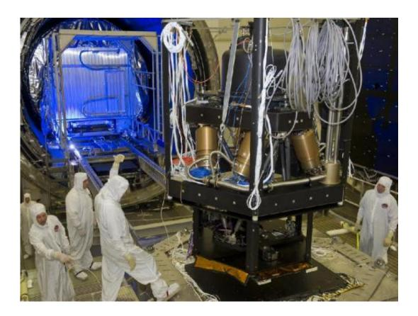
NASA's Marshall Space Flight Center in Huntsville, Ala., recently completed testing of COCOA. The work was done in the X-ray and Cryogenic Test Facility. The optical assembly was operated in a vacuum at both room temperature and cryogenic -- or deep cold -- temperatures to certify its performance before it is used to test the performance of Webb's 21.3-foot primary mirror. Credit: NASA Marshall
