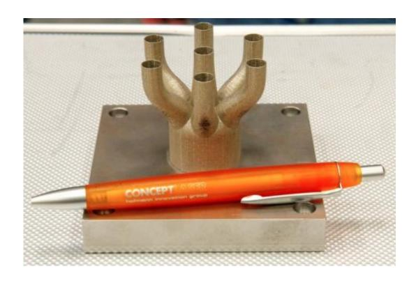
First test piece produced on the M2 Cusing Machine at the Marshall Center. Credit: NASA/MSFC/Andy Hardin
