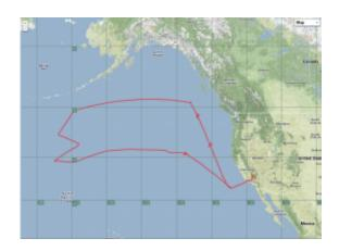
The Global Hawk departed from NASA Dryden on Nov. 6 and flew along the Pacific Coast to as far north as Washington state. During the 24.2-hour flight, the aircraft flew over four Pacific Ocean buoys and a low-pressure system south of the Aleutian Islands in Alaska. Credit: NASA
