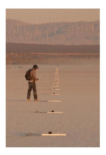
A FaINT project researcher adjusts one of the microphones in a linear array nearly 1 ½ miles long laid out by the project team to record and measure sonic booms. Credit: NASA/Tom Tschida
