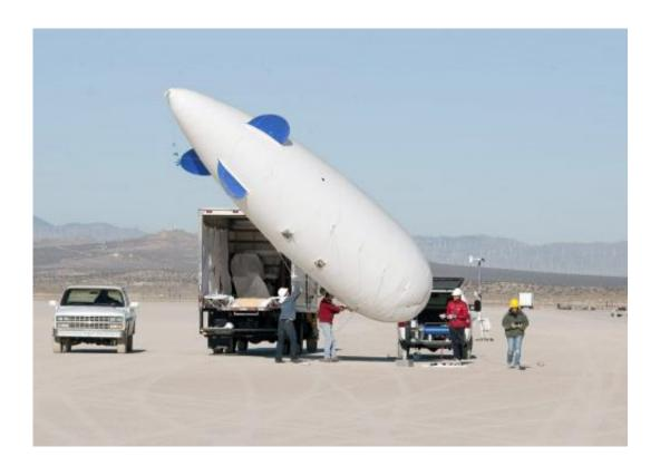
Cessna researchers prepare to launch a blimp that carries several microphones used to record sonic booms for the FaINT project. The tethered blimp flies at an altitude of about 3,000 feet above ground to collect sonic boom data at that altitude. Credit: NASA/Tom Tschida
