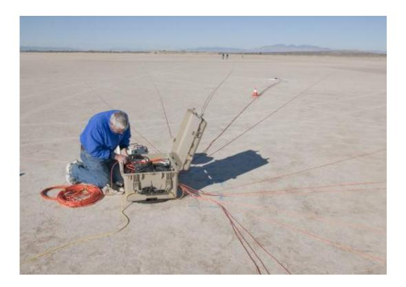
Like being in the center of a giant orange spider web, a FaINT project researcher connects microphone wiring for a spiral array designed to collect sonic boom data for the project. Credit: NASA/Tom Tschida
