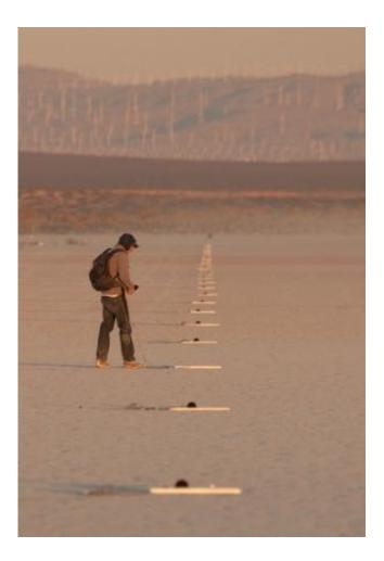
A FaINT project researcher adjusts one of the microphones in a linear array nearly 1 ½ miles long laid out by the project team to record and measure sonic booms. Credit: NASA/Tom Tschida
