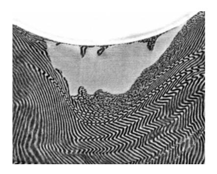
This electron-microscope image of a cross-section of a layered polymer shows the crater left by an impacting glass bead, and the deformation of the previously even, parallel lines of the layered structure as a result of the impact. In this test, the layered material was edge-on to the impact. Comparative tests showed that when the projectile hit head-on, the material was able to resist the impact much more effectively. Credit: Thomas Lab, Rice University
