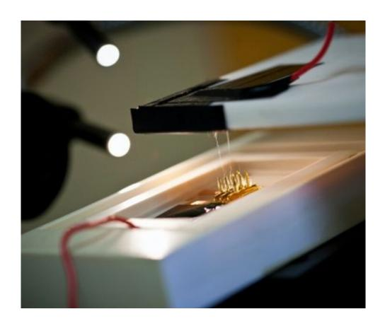
A tiny array of silicon tips sandwiched between electrodes spins out "nanofibers" of plastic that could be useful for a host of applications. Credit: Dominick Reuter
