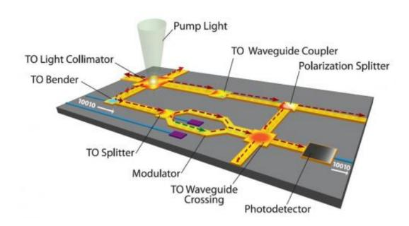
Transformation optics devices that perform diverse, simple functions can be integrated together to build complex photonic systems for optical communications, imaging, computing, and sensing. Credit: Qi Wu
