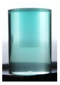
The research team developed a detector to measure the radiation dose in three dimensions.
