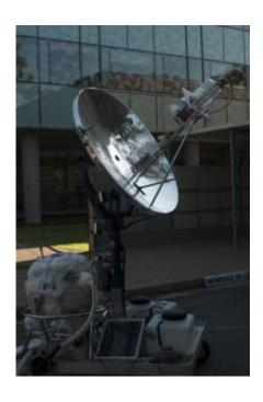
New solar steam technology developed at Rice University uses nanoparticles so effective at turning sunlight into heat that it can produce steam from icy-cold water. Credit: Jeff Fitlow/Rice University
