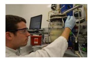
UC Berkeley graduate student Zachary Baer works with a fermentation chamber to separate acetone and butanol (top clear layer) from the *Clostridium* brew at the bottom. The chemicals can be extracted and catalytically altered to make a fuel that burns like diesel. Credit: Robert Sanders
