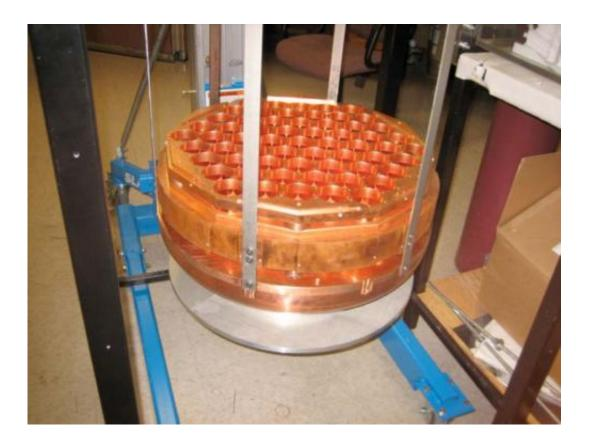
Shown is a side view of the Lawrence Livermore National Laboratory-designed and built copper photomultiplier tube mounting structure, which is a key component of the Large Underground Xenon (LUX) detector, located at the Sanford Underground Research Facility in Lead, S.D.
