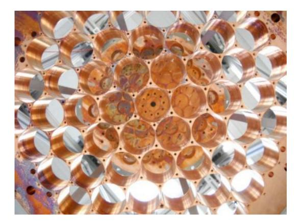
Shown is a top-down view of the Lawrence Livermore National Laboratorydesigned and built copper photomultiplier tube mounting structure, which is a key component of the LUX detector.
