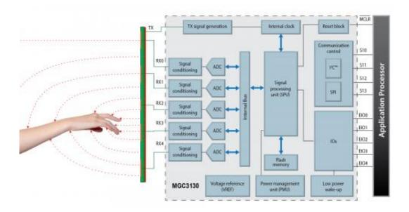
The company is offering a development kit. A gesture library was constructed using algorithms that learned from how different people make the same movements, to be applied toward device functions such as .point, click, zoom, or scroll. Ten gestures were programmed into the device with recognition based on Markov models. According to the company, "the chip provides developers the flexibility to utilize prefiltered electrode signals for additional functionality in their applications."
