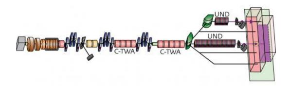
The principle of SACLA. The laser consists of various electron acceleration stages (C-TWA) and focusing elements. Key to achieving short wavelength operation is, however, the design of the undulator (UND). Credit: 2012 Nature Publishing Group
