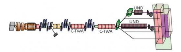
The principle of SACLA. The laser consists of various electron acceleration stages (C-TWA) and focusing elements. Key to achieving short wavelength operation is, however, the design of the undulator (UND). Credit: 2012 Nature Publishing Group
