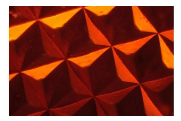
This is a microscopic image of a silk optical implant treated with the cancer fighting drug doxorubicin. When implanted in tissue, the mirror released a controlled dosage of the drug as it gradually dissolved. The amount of reflected light decreased as the mirror degraded, allowing the researchers to accurately assess the rate of drug delivery. Credit: Fiorenzo Omenetto
