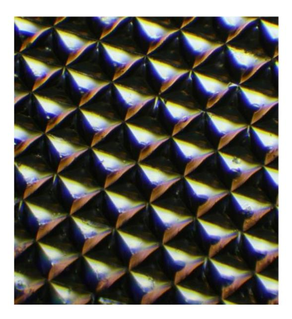
This is a microscopic image of a silk optical implant created when purified silk protein is poured into molds in the shape of multiple micro-sized reflectors and then air-dried. When implanted in tissue and illuminated, the "silk mirrors" caused more light to be reflected from within the tissue allowing for enhanced
