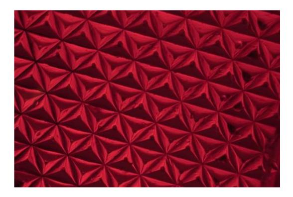
This is a microscopic image of a silk optical implant embedded with gold nano particles. When implanted in tissue and illuminated with green laser light, the particles converted light to heat, turning the reflector into a thermal therapy to control bacterial infection or kill malignant cells. The implant's optical capabilities allowed researchers to monitor the progress of the therapy. Credit: Fiorenzo Omenetto
