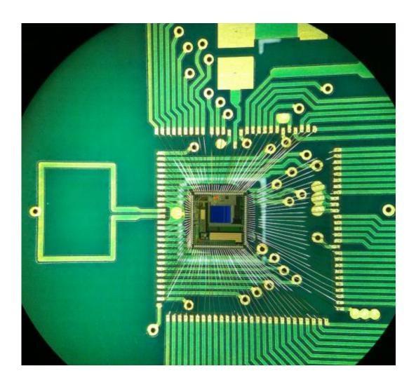
A close-up of the new chip, equipped with a radio transmitter, which is powered by a natural battery found deep in the mammalian ear. Credit: Patrick P. Mercier
