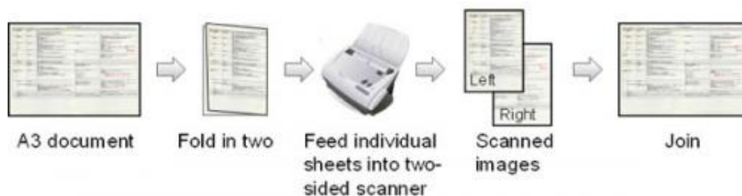
Figure 1: Conventional method for scanning A3 documents with A4-size scanner.
