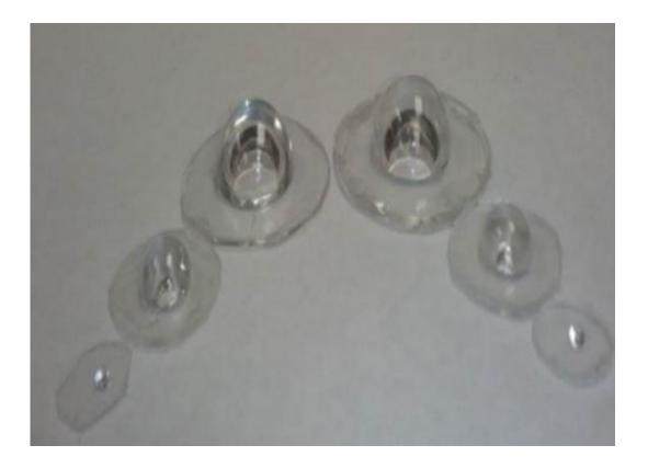
These light-gathering polymer lenses are 3.5 times more powerful than glass, and are the first commercial nanolayered product to come out of many years of R&D at Case Western Reserve University. To create the lenses, a 4,000-layer film is coextruded, and then 200 layers of film are stacked to create an 800,000-nanolayer sheet. Credit: Photo courtesy Michael Ponting.
