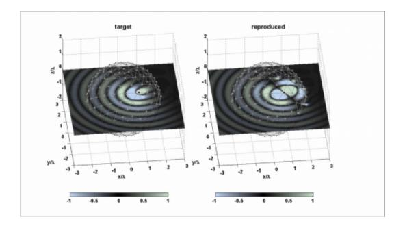
This shows a sound field reproduced from a sound ball. The left is a target sound source, and the right is a virtual sound source (sound ball) created by loudspeakers. Credit: KAIST Acoustics & Vibrations Lab
