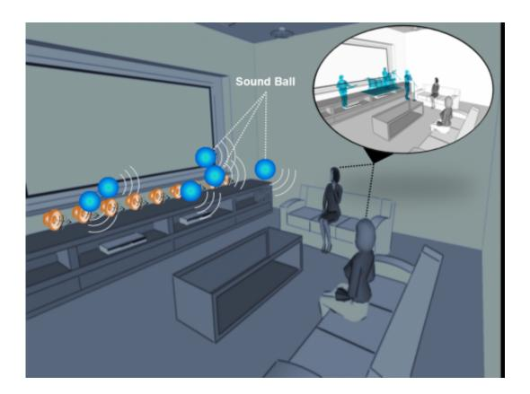
The sound ball system is a technology that installs virtual speakers by utilizing multiple loudspeakers to concentrate acoustic energy temporally and spatially into a spot where the loudspeakers do not exist physically. The virtual speakers then reproduce a desired sound field perceived by the listener. Credit: KAIST Acoustics & Vibrations Lab
