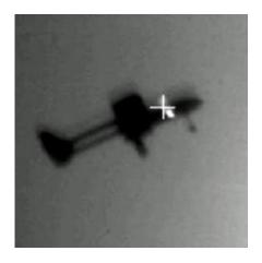
Sensor image shows engagement by the ADAM system of an unmanned aerial system target.
