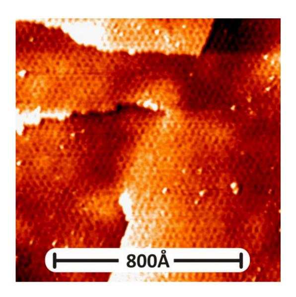
Scanning tunneling microscopy shows the topography of graphene on gold with periodic beatings ten times larger than the periodicity of the carbon atoms. These beatings are moiré-patterns, emerging because of the different atomic structures of graphene and the underlying monolayer of gold atoms. The structure of moiré
