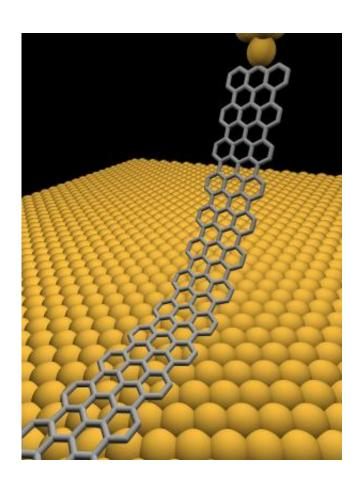
Electric circuit with nanocable: Max Planck researchers from Berlin lift a graphene ribbon from a gold surface with the tip of a scanning tunnelling microscope and investigate how the conductance of the carbon ribbon depends on its length. Credit: Leonhard Grill / Fritz Haber Institute of the Max Planck Society
