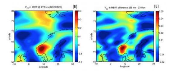
The image on the left shows GOCE's gravity measurements over northern Europe, acquired from its previous altitude. The image on the right depicts the expected measurements over the same area after the satellite has been lowered by 15 km. An increased signal and improved spatial resolution is evident. Credit: ESA / GOCE+ Theme 2
