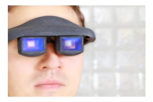
Users can control the display of these data glasses with their eye movements. Credit: Fraunhofer COMEDD
