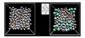
Making glass by changing the structure of a liquid. Left: normal liquid alloy of nickel (silver) and phosphorous (orange) atoms. Encouraging atoms to form bicapped square antiprisms (inset) turned the liquid into a solid glass (right) where the nickel (turquoise) and phosphorous (green) atoms in antiprisms are drawn larger
