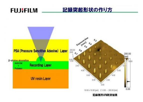
The structure of the two-photon absorption material (left) and the variation of the convex shape depending on the irradiation time of a laser light (right). Credit: TechOn!
