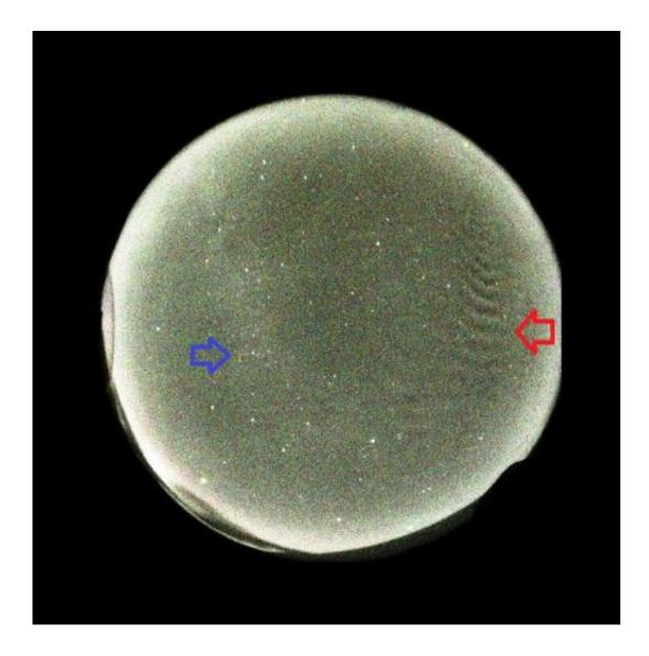
The red arrow points to the unidentified low-intensity wave pattern, which the researchers suspect is an auroral-generated wave interaction with airglow. For contrast, the blue arrow points to the faint emission of the Milky Way. Credit: *Optics Express*
