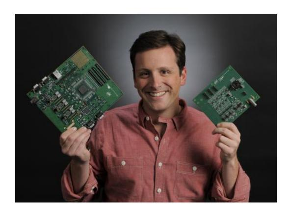
Goddard technologist Jonathan Pellish holds a Goddard-developed digital test board (larger) and the IRAD-developed daughter card containing the analog-based data-processing integrated circuit. The daughter card snaps into the digital test board and will be used to test a number of spaceflight processing applications. Credit: NASA/Goddard/Pat Izzo
