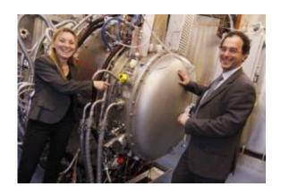
Ready: IPP's new ion source (far right), incorporated in the just completed ELISE test rig. The door-sized particle beam produced here is to transport the immense power of 1.2 megawatts. The rest rig was officially commissioned on 27 November 2012 by Professor Ursel Fantz of IPP and Dr. Antonio Masiello of "Fusion for Energy" (Photo: IPP, Robert Haas).
