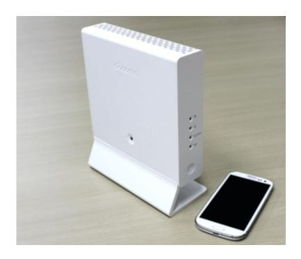
DOCOMO's new small-cell base station supporting 3G and LTE.
