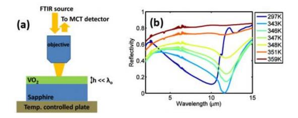
Left: This diagram shows the experimental setup used for measuring the reflectivity of the vanadium-sapphire device. The vanadium oxide layer is only 180 nanometers thick, much thinner than the wavelength of the incident infrared light. Right: At just the right temperature (light blue line), the reflectivity of the device drops almost to zero (99.75 percent absorbance) for infrared light at a wavelength of 11.6 microns. Credit: Mikhail Kats.
