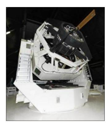
DARPA's ground-based <u>Space Surveillance Telescope (SST)</u> may soon head to Australia. An agreement reached this week with Australia's Department of Defense will allow DARPA to take the 180,000 lb. threemirror Mersenne-Schmidt telescope to Australia to track and catalogues
