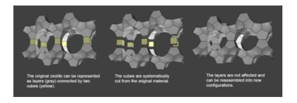
Researchers from Leuven, Ghent and Antwerp have now experimentally demonstrated that it is possible to cut zeolite building blocks and rearrange them into a new structure. Professor Christine Kirschhock of KU Leuven explains: "A zeolite can be thought of as a set of merged building blocks. We are now able to separate certain blocks of a zeolite and then reassemble them into different configurations, depending on
