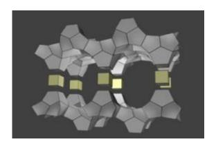
The original zeolite can be represented as layers (gray) connected by cubes (yellow). The new method systematically cuts the cubes from the original material allowing the layers to be reassembled into new configurations.
