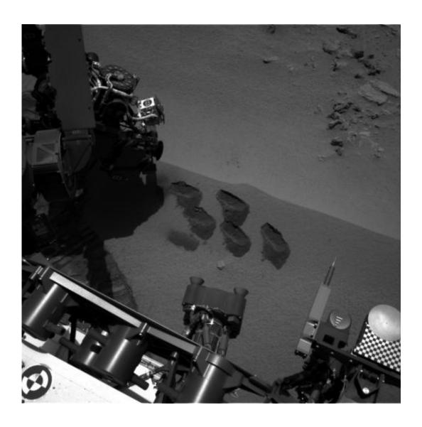
NASA's Mars rover Curiosity used a mechanism on its robotic arm to dig up five scoopfuls of material from a patch of dusty sand called "Rocknest," producing the five bite-mark pits visible in this image from the rover's left Navigation Camera (Navcam). Each of the pits is about 2 inches (5 centimeters) wide. The
